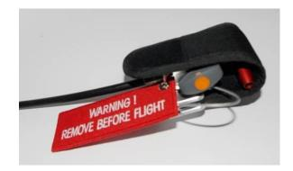
Before the flight you have to take the key out and to give on its place the safety "Quick pin".
