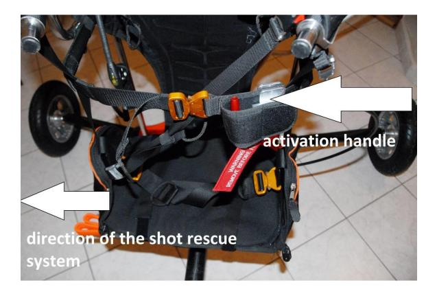
By the installation of the ballistic rescue system take care that the rocket engine pulls out the parachute to the side of the hand by which you will activate the rescue system. Raising the hand to the activating handle of the rescue system you will free the area before the rocket engine and prevent a possible injury, that it could cause to you. The most suitable place for the rescue system is by the motor paragliding under the seat. Any installation must be consulted with the producer!
