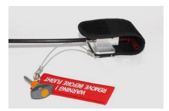
After the start you must push out in the shortest time the safety "Quick pin"!
