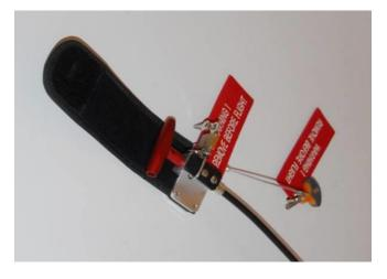
The rescue system must be during the time, when you do not fly with it, secured by the key delivered by the producer. This together fulfilles the function of the transport safety catch.
